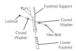
FIGURE 6.4 Footrest Height Adjustment - 70° and PW93
